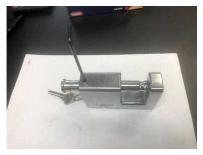
Using 1/8 hex key remove grub screw.
