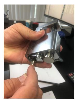
Remove key from cylinder. With padlock keyway facing down press onto cylinder to remove shroud.
